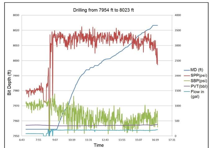
Figure 5. Drilling Operating Parameters up to 8023 ft.
