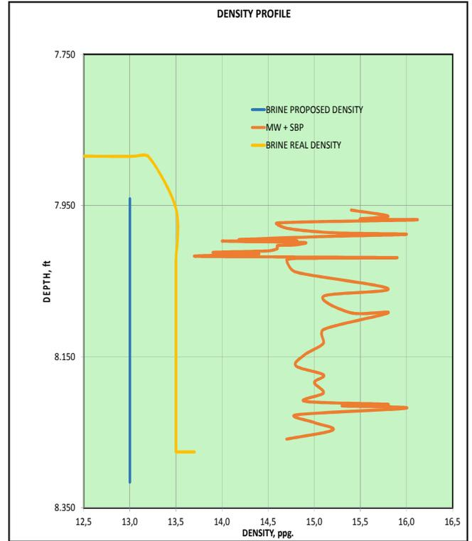
Figure 2. Density Profiles of the proposed versus actual field conditions.
