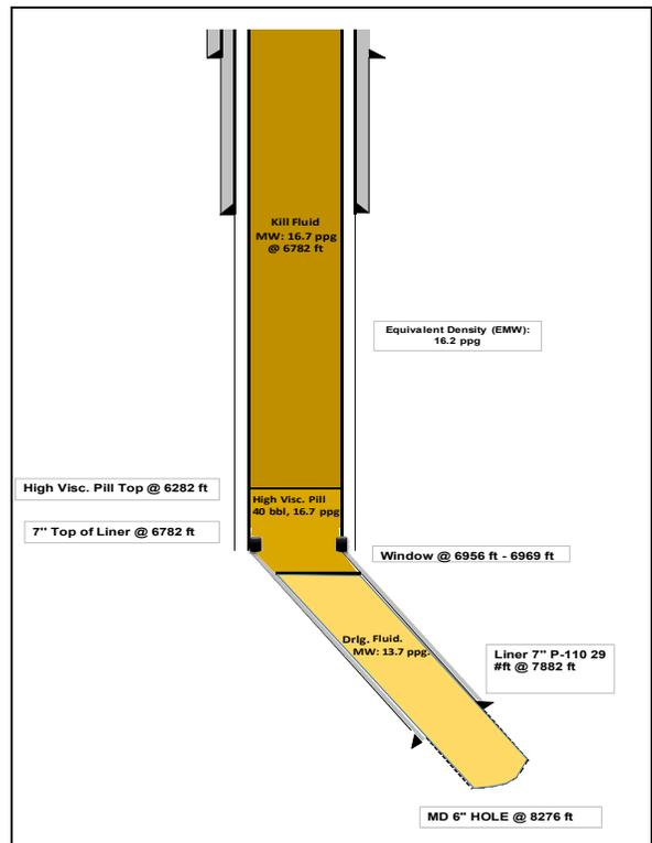
Figure 8. Density Profile proposed for well control.
