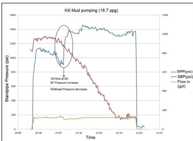
Figure 9. Operating parameters during well control.
