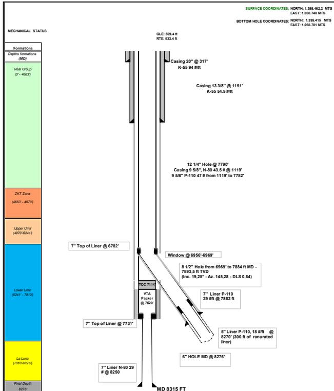
Figure 1. Mechanical Status of the Well.
