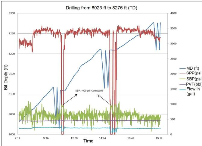
Figure 6. Drilling Operating Parameters up to TD.
