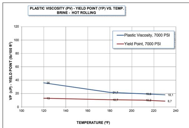
Figure 3. Drilling Fluid HPHT<sup>4</sup> Rheology.
