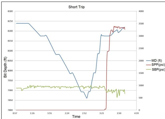
Figure 7. Drilling Operating Parameters – Short Trip to the Shoe.
