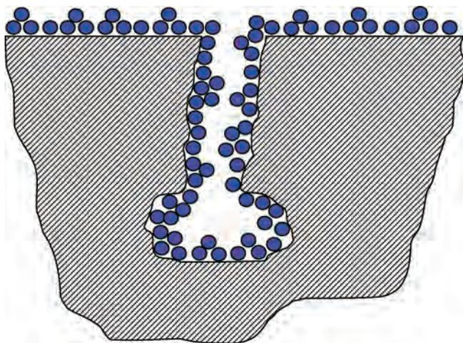
Fig. 3—Methane molecules adsorbed onto a cleat network of coal.
