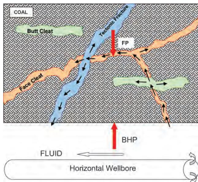
Fig. 8—BHP enters the face cleat, and dissipates over time through the fracture network to equal the FP. No barrier exists to prevent the equalization of BHP and FP.
