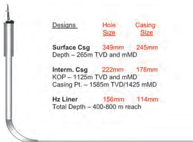
**Fig. 10—Generic wellhole/casing design for coalbed methane wells drilled.**
