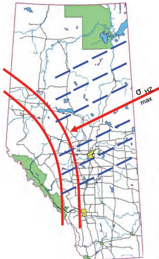
Fig. 5—Map of Alberta showing stresses and cleating. Preferred orientation of the face cleats (blue lines), in a NE/SW direction, which is the same direction as the principle horizontal stress  $\sigma_{Hz\ max}$ . Front line of the Rocky Mountains (curved red lines). The majority of the Mannville horizontal CBM wells have been drilled in a NW/SE direction.
