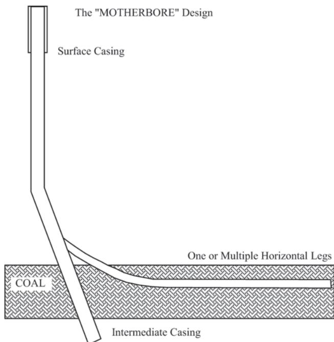
**Fig. 6—“MOTHERBORE” design in which multiple legs are possible from one central casing string.**
