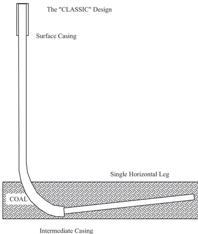
**Fig. 7—“CLASSIC” CBM horizontal wellbore design with a single horizontal leg, which is often slightly inclined to assist in drainage of water during the production phase.**
