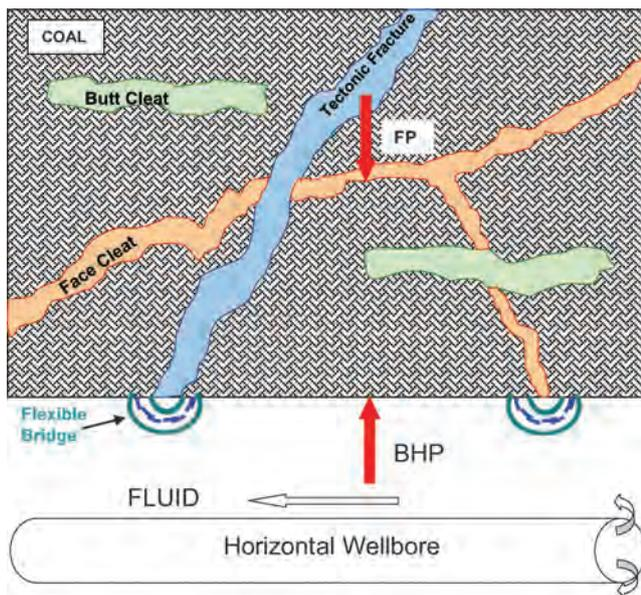
**Fig. 9—Flexible bridge/mat is formed across the face cleat and tectonic fractures, thereby preventing fluid/pressure penetration. BHP is maintained higher than the FP, with resulting borehole stability and decreased formation damage.**
