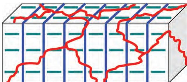
Fig. 1—Stylized depiction of a coal showing the face cleats (blue), butt cleats (green), and tectonic fractures (red).
