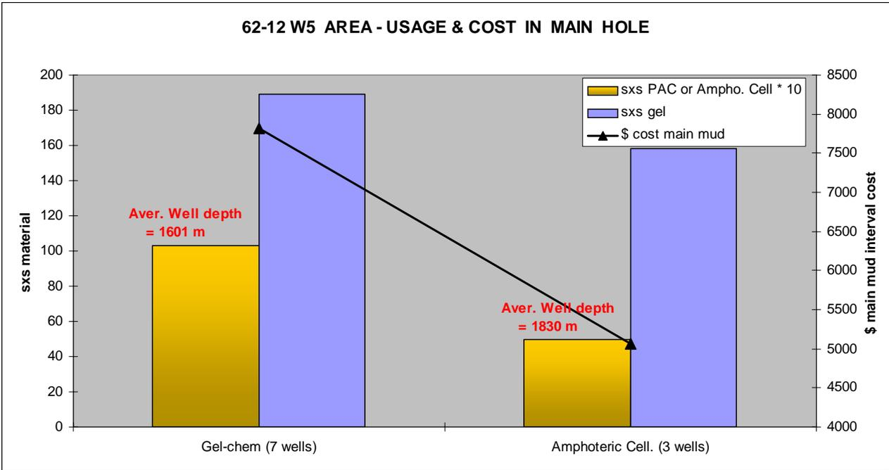
**Figure 4: Average Main Hole Material Usage and Interval Costs for Gel-chemical and Amphoteric Cellulose Wells. Material Usage are in “bars” and Costs are Depicted by the Line. Note that sxs of PAC or Amphoteric Cellulose Material are Multiplied 10 fold.**
