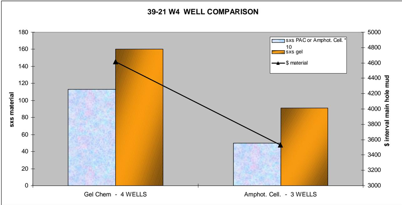
Figure 2: Average Main Hole Material Usage and Interval Costs for Gel-chemical and Amphoteric Cellulose Wells. Material Usage are in “bars” and Costs are Depicted by the Line. Note that sxs of PAC or Amphoteric Cellulose Material are Multiplied 10 fold.
