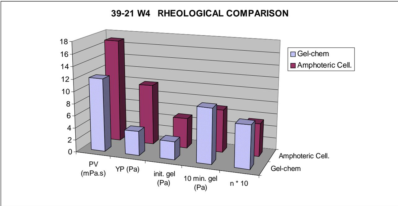
Figure 3: Average Rheological Data for Gel-chemical vs. Amphoteric Cellulose Ether Mud System Comparison.
