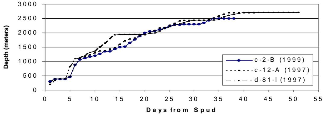
Fig 4. – Depth/Days Progress Curves for c-2-B, Silicate Well, and most Recent Offset Wells. The Offset Wells were Drilled with Gel-PHPA Drilling Fluids and had Intermediate Casings Strings set at 2436 m (c-12-A) and 2444 m (d-81-I).
