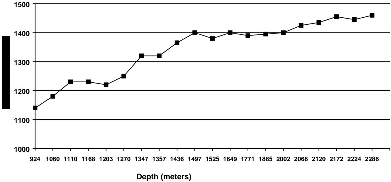
Fig 6. – Plot of Drilling Fluid Density with Depth in the Intermediate Hole Section of c-2-B. Very Sharp Gas Kicks were Noted at 1051 meters, 1261 meters and 1296 meters. High Connection Gas and Background Gas was Observed from 1296 meters to Casing Point.
