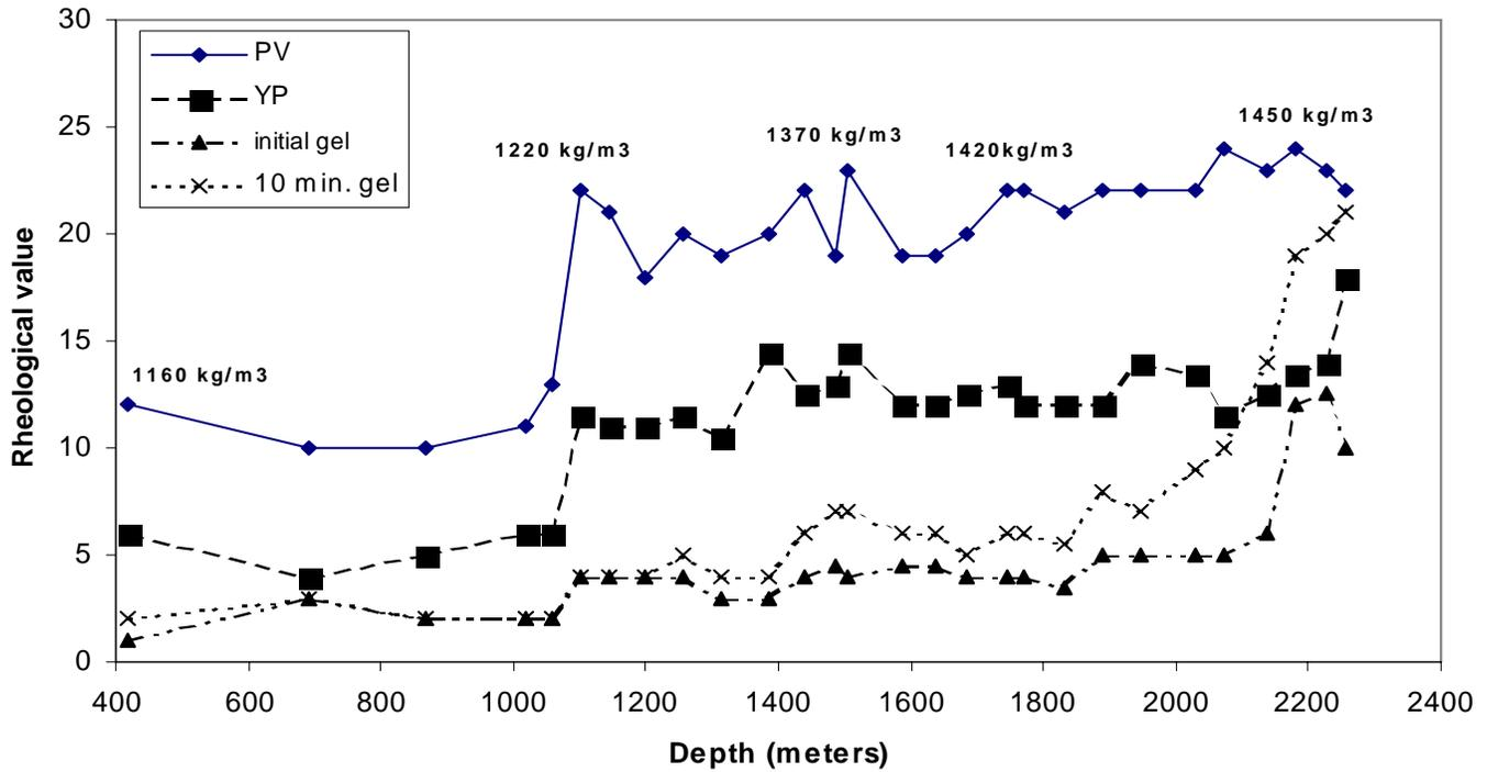
**Fig. 8 – Comparison of Rheological Parameters of Silicate Drilling Fluid in Intermediate Section of c-2-B Well. Increases in Density to Control Gas Influxes Increased Rheological Values. The Sharp Increase in YP and Gels near TD was Planned in Preparation for Running Logs. PV is Plastic Viscosity (mPa.s), YP is Yield Point (Pa), gel strengths are taken after 10 seconds and 10 minutes (Pa).**
