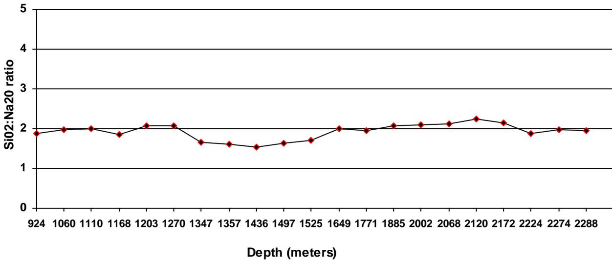
Fig. 7 – SiO<sub>2</sub> and Na<sub>2</sub>O Ratio Maintained in Drilling Fluid at c-2-B while Drilling Intermediate Section. Ideal ratio of 2.0 was Consistent through the Section Except during the 1350-1649 meter Interval.
